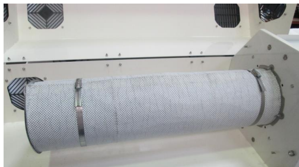
Internal TiO 2 /activated carbon filter
