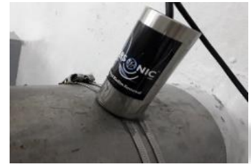
TD50grip with SS strap of 70mm Stan cable 10m (131300.198 xlr / 156337.198 no xlr) OR EMC cable (10m 146901.198 / 25m 157347.198)
